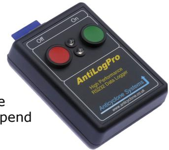
Hold the 'On' button down until a green LED lights and then release will put the unit in playback menu mode. Playback menu mode allows you to configure your unit using an easy to use terminal menu system. Recorded data can be replayed or upload to a PC, Laptop or other host machine of your choice. Data can even be played back in real time on up to two RS232 output channels simultaneously to simulate real equipment output.
