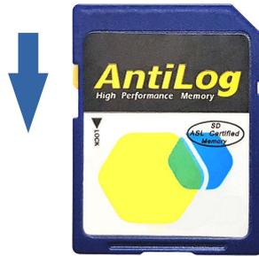
Figure 1: Setting the media lock switch
